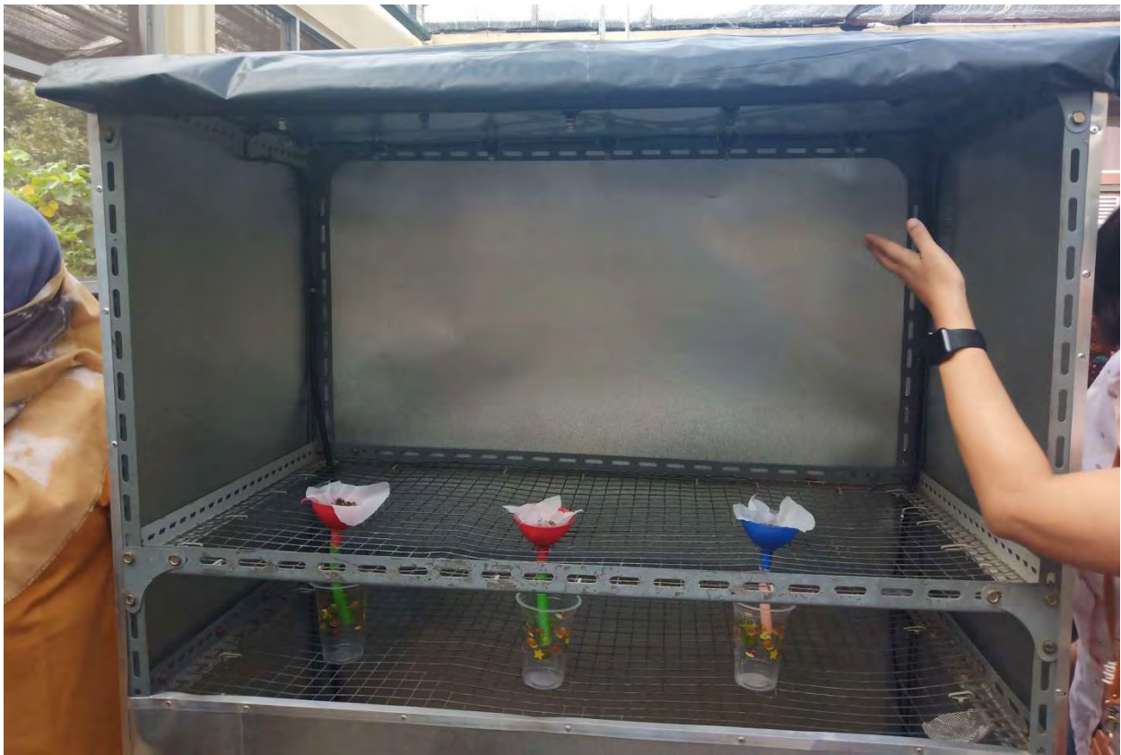
Photos 12. Participants performing the sucrose-centrifugation method and preparation of sucrose solution for extracting potato cyst nematodes from infested soil (above). Improvised mist chamber set-up for extracting nematodes from soil and root substrates. This method was demonstrated during the laboratory practicals (below).
