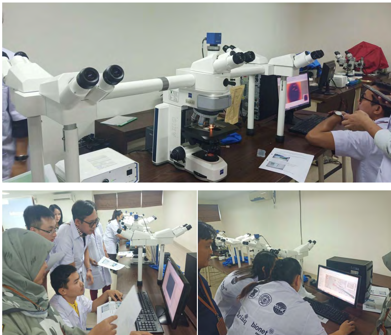
Photo 18. Multi-channel compound microscope with 5-paired eyepiece and attached to a computer for morphometrical analysis and photo documentation of nematodes (above). Participants while performing the actual measurements of nematode body parts for morphological identification (below).
