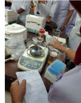
Centrifuge tubes need to be in equal weight
