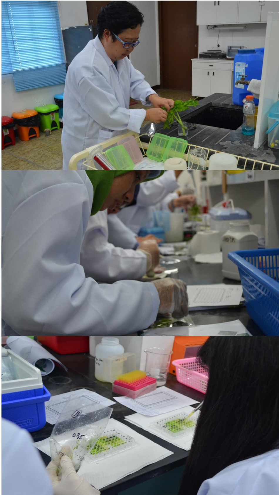
Fig. 31. Extraction of plant samples and loading of extracts into ELISA plate for incubation.
