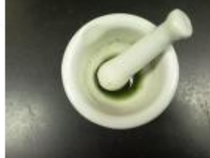
3 Grinding the sample with General Extract Buffer (GEB)
