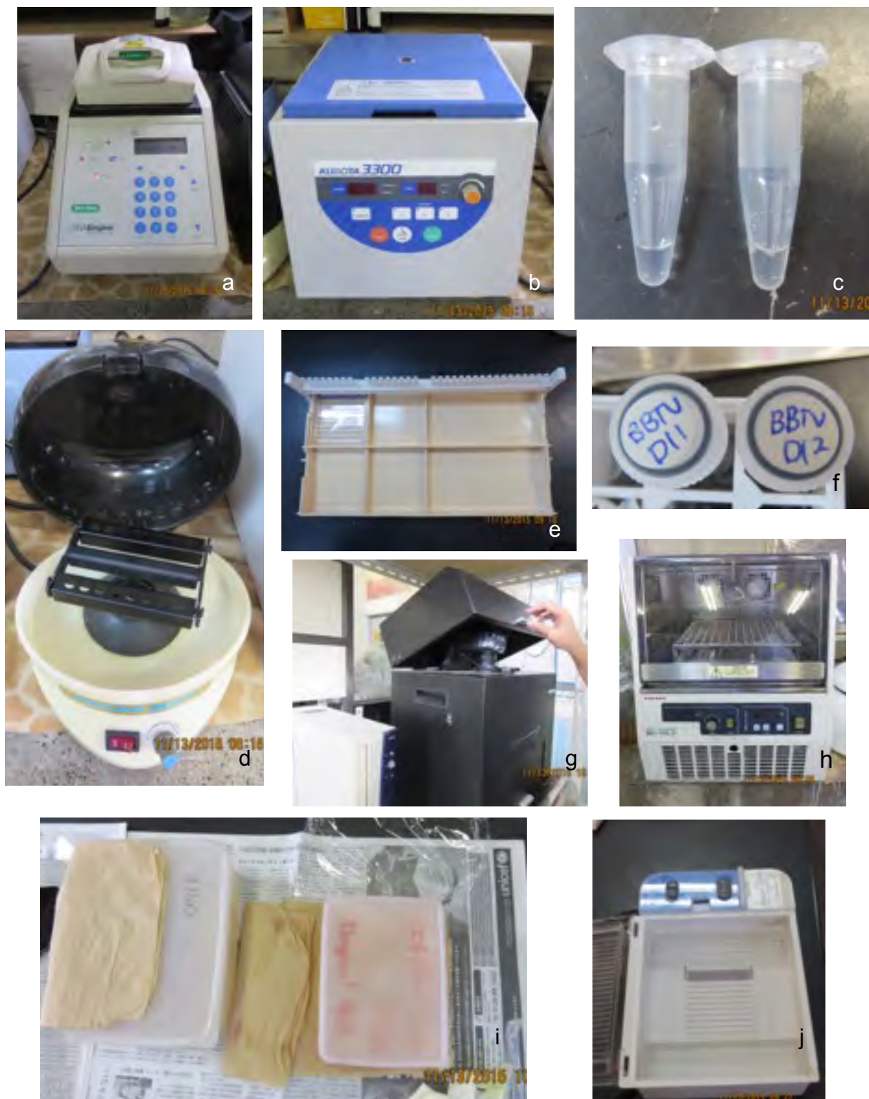
Figure 2: Equipments used for the DNA extraction, PCR amplification and gel electrophoresis. (a) thermocycler; (b) centrifuge; (c) 1.5 mL micro centrifuge tube containing extracted DNA; (e) gel case and comb; (f) primers for BBTv; (g) UV illuminator with camera; (h) shaker; (i) containers containing EtBr and distilled water; (j) gel electrophoresis
