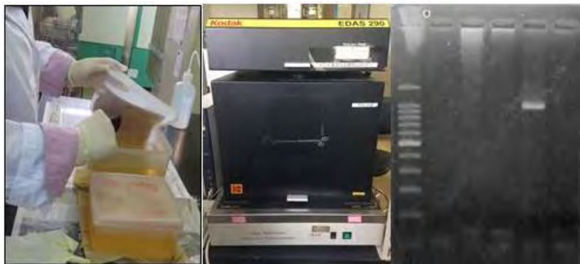
Fig. 9: Gel staining with EtBr and viewing of DNA band under UV transilluminator
