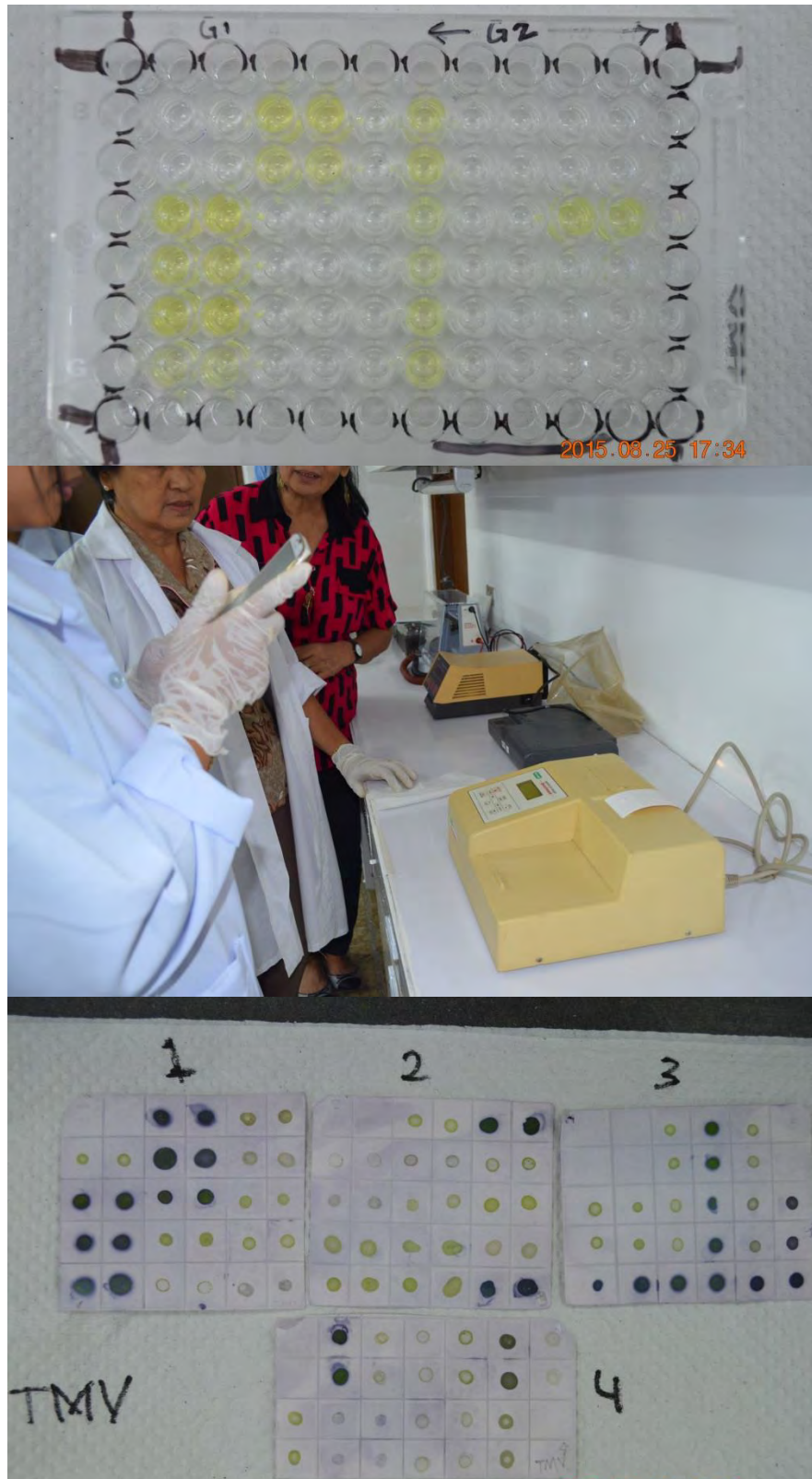
Fig. 34. Color observation of ELISA results (upper) and reading of the absorbance value using ELISA reader (middle). Visual observation on DIBA was also performed during day 8 of laboratory exercise (lower).
